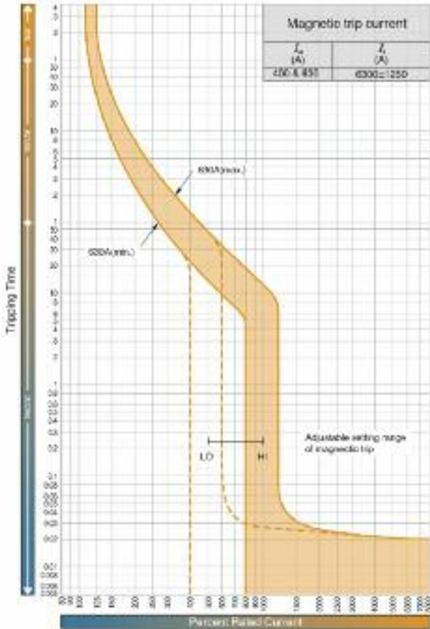
YA6 Time/Current Curve (Thermal / Magnetic 400A-630A)
