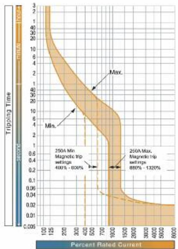
YB3N & YB3S 3 and 4-pole Time/Current Characteristics for 250A
