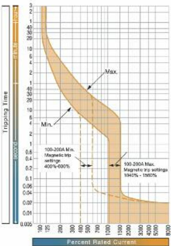
YB3N & YB3S 3 and 4-pole Time/Current Characteristics up to 200A
