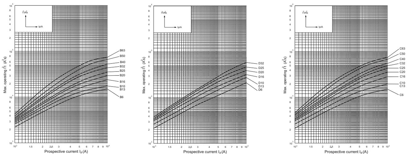
The following table indicates the maximum energy let-through values permissible in each class, stated in Watt-seconds. In practice, compliance with the standard is checked on the circuit breakers with the highest applicable rated current within the range, normally 40A.
