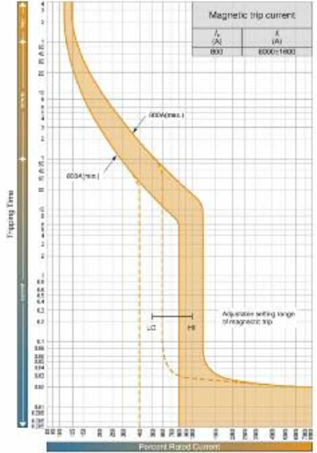
YA6 Time/Current Curve (Thermal / Magnetic 800A)
