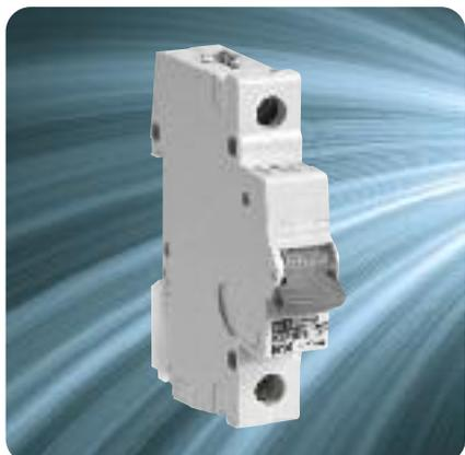
These devices are used to provide protection and control of circuits against overload and short circuit conditions. Dorman Smith MCBs are supplied with various breaking capacities, particularly for ratings of 6kA and 10kA. The lower rated devices are used typically in domestic installations, e.g. in consumer units, whereas the higher rated devices are suitable for a range of commercial and industrial circuit protection applications.
